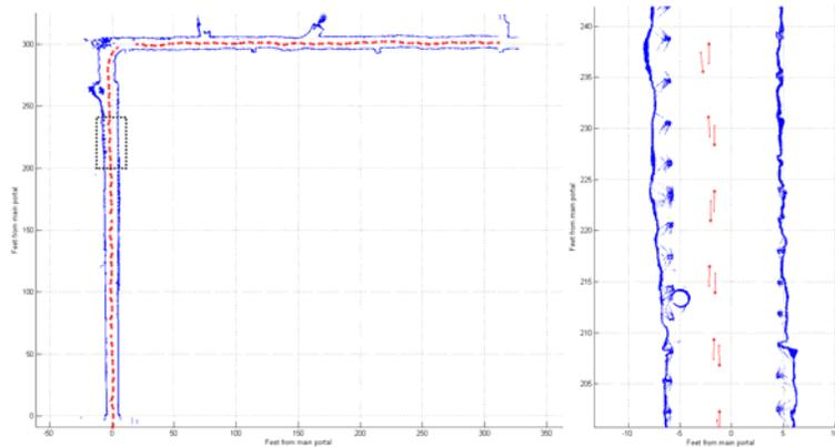
**Figure 4: Scan Coverage. (Left)** This map is actually a thin slice of data extracted from a robotically generated model. This model contains 172 individual LIDAR scans that were fused from 86 robot stations covering 183 meters of mine corridor. **(Right)** A magnified view of this map showing a 12m section of corridor. The arrows in the center of the map show the position and heading of each LIDAR scan.
