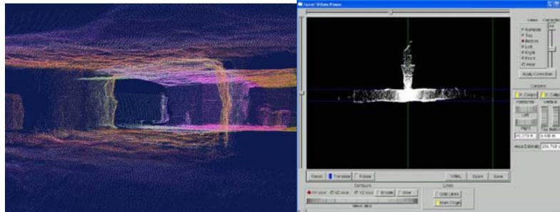
**Figure 6: 3D Data Manipulation.** (Left) A limestone mine model is visualized by coloring each individual scan with a random color. This model can be flown-through, meshed or cut into cross sections as needed. (Right) Analytical tools provide measurements from subterranean models in the form of cross sections, area and volume calculations.
