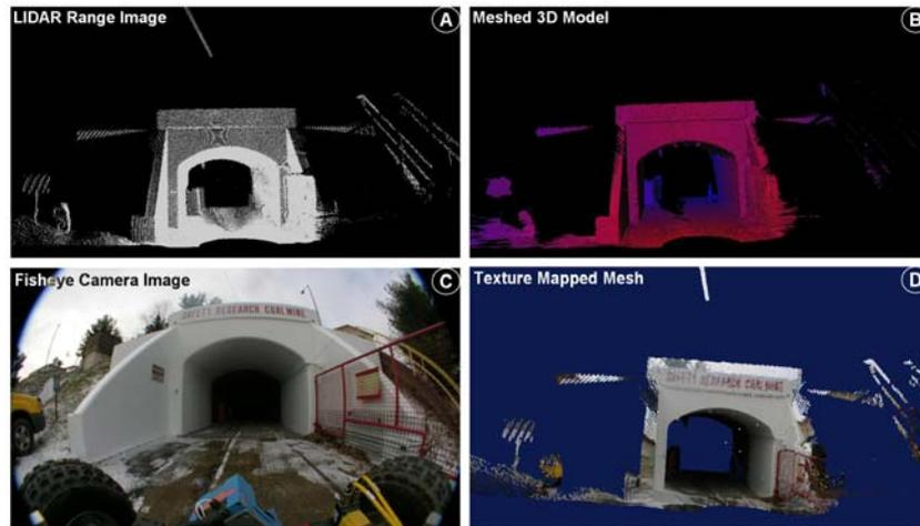
Figure 3: Production of a texture-mapped mesh. (A) Raw LIDAR data is visualized as a point cloud whereas in Fig. 2, it was shown as a data stream. (B) A surface (or mesh) is applied to the point cloud. (C) A fisheye image of the scene is taken during capture of the LIDAR image. Note: the LIDAR sensor is visible at the bottom of the photograph. (D) Image pixels paint the mesh to produce the final textured-mapped model.
