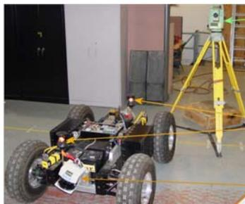
**Figure 1: Combined survey instrument and mobile robot.**
