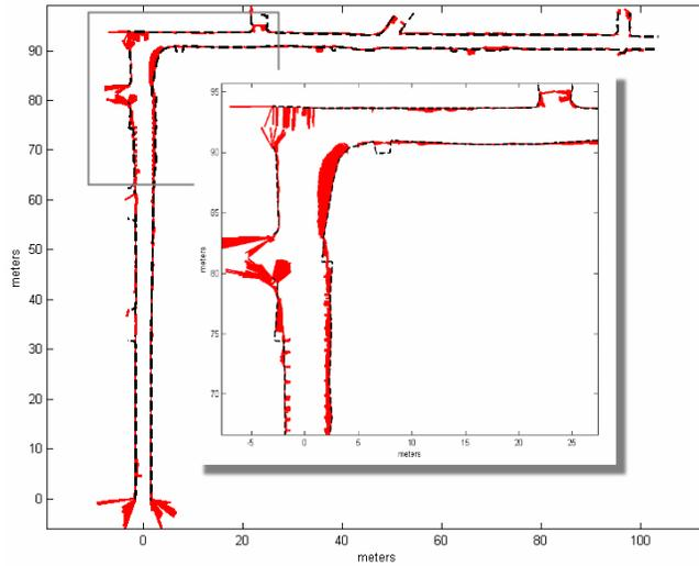
**Figure 5: Map Comparisons.** The original mine map is represented by the dashed line. Differences between the prior and robot-generated maps are signified by the colored area surrounding the dashed line. The robot-generated map remains consistent to the “idealized” mine map; however, locations where mine interior has changed are distinguishable.
